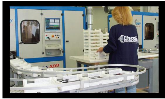
Two MEI robotic edgers (a Bisphera XDD and a Double R-XDD) in the finishing department are fed by automatic conveyors.
