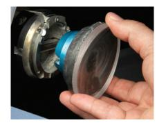
house lens production. Based on Gerber Coburn's full-scaled DTL generator, the CTL provides a smaller scaled model at a low cost of entry into free-form production but with the ability to grow with the needs of the lab.
